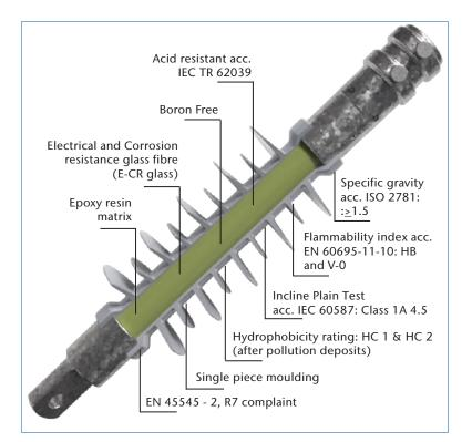
Designed and Tested according to: EN 50119 EN 50124 EN 62621 EN 61109 The HTV<sup>1</sup> housing is of overmoulded design and moulded in a single piece. It encapsulates the triple point (meeting of end fitting, silicone and core rod) making the interface impervious to moisture.
