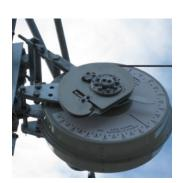
By means of a support cable, TENSOREX C+ exerts a constant tension on the contact wire, regardless of any changes in force due to temperature. The special spiral spring is firmly connected to a shaft which are firmly connected both cams/pulleys.
