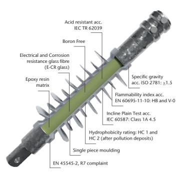
Designed and tested according to: EN 50119 EN 50124 EN 62621 EN 61109 EN 61952 EN 62217
