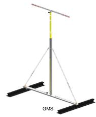
This measuring device measures the height and stagger of the contact wire with different rulers fixed in the mast.
