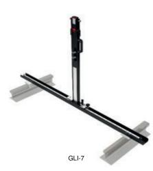
This measuring device uses a laser rangefinder to measure the height and stagger of the contact wire. Some versions can also be used for inclination measurement and for measuring the distance to the mast.
