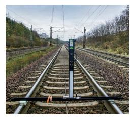
The Mosdorfer Rail catenary geometry laser measuring device combines ease of operation with maximum precision in
