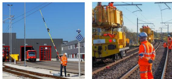
Safety equipment is one of the most sensitive aspects of railway electrification. Reliable products, ease of use and operational safety are therefore essential. Mosdorfer Rail offers a complete range of voltage detectors, earthing and operating poles, which can be exactly match to any requirements thanks to our modular system design.
